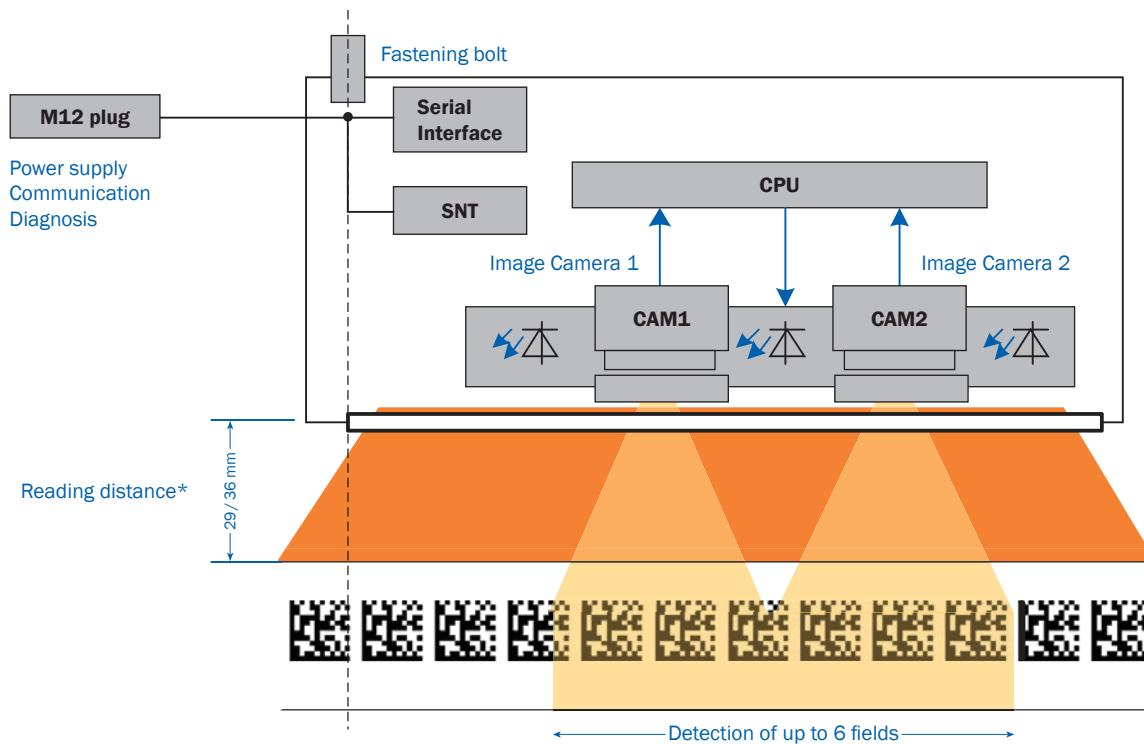
The positioning system operates with the simple and efficient Data Matrix code strip. This permits absolute position detection up to a maximum travel range of 10.000 meters. Instant positioning is available after interruptions and the LED light source is unaffected by ambient lighting conditions.
