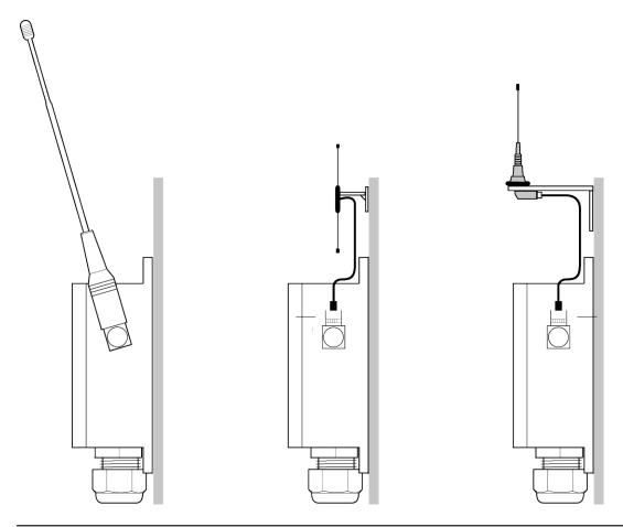
NOTE! For optimum performance: Place well away from metal objects, such as metal girders, highvoltage cables and other antennas.
