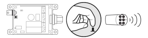
The receiver can be programmed to accept up to 15 different transmitters for relay 1 and up to 15 different transmitters for relay 2. Each transmitter has a unique ID code.
